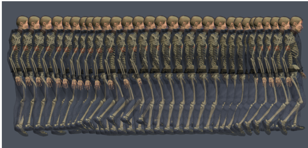
Figure 3.7: Once the semi-automatic skeleton alignment was completed on the initial pose, an animation for Ralph was loaded to further look for penetrations with the mesh of Ralph, i.e. if the skeleton was fully contained. As a visual aid, an extra widget was added to RAGE's GUI to interactively change the transparency of Ralph's mesh in OGRE. The above figure shows an animation history plot of Ralph loaded with a walk-cycle animation and Ralph's mesh transparency set to 50%.
